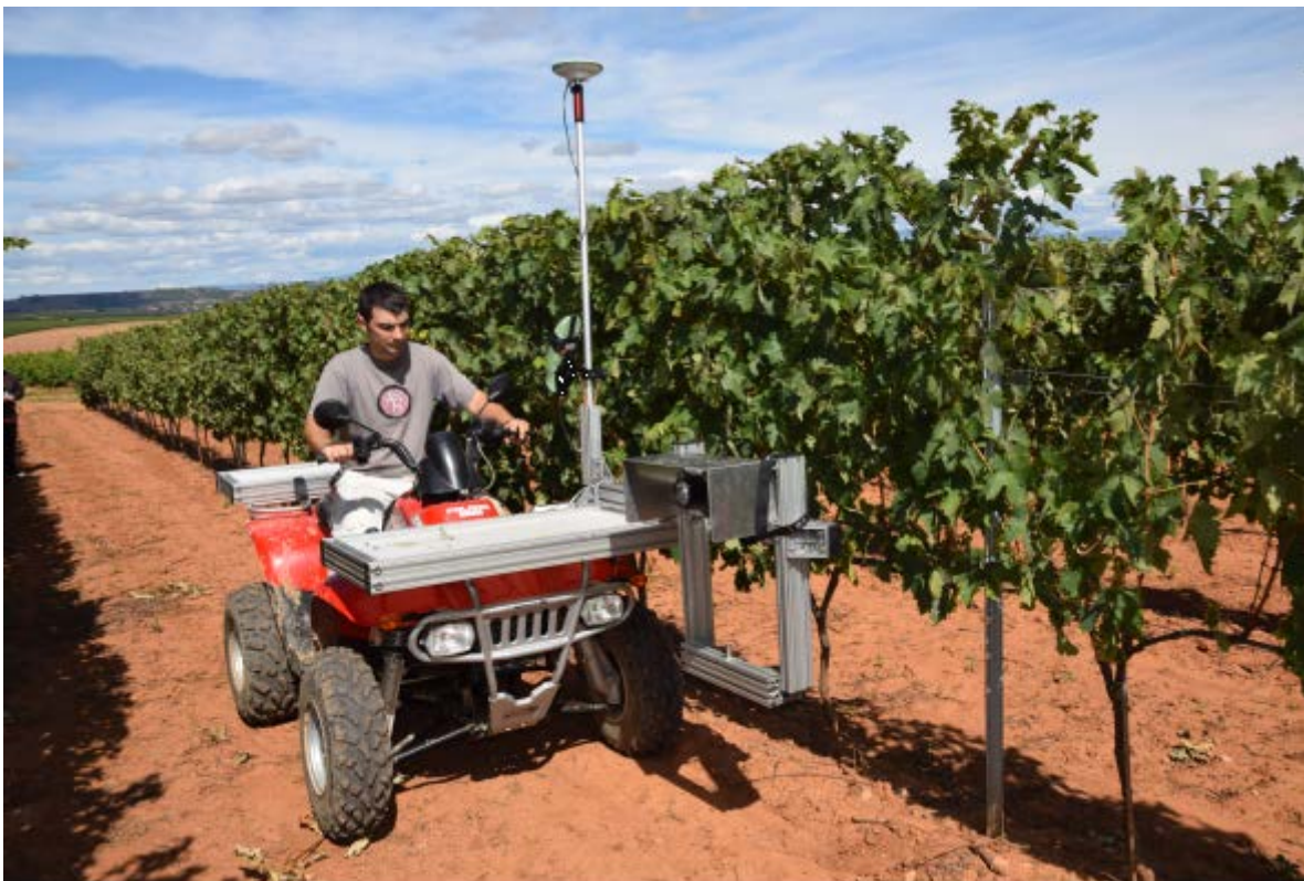
Figure 1: Modified ATV for automatic image capture on-the-go. Equipped with a GPS antenna LED Light Panel, RGB camera and inductive sensor for camera triggering (3 pulses per revolution).
